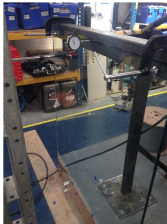
Figure 2: Setup for MS123 during horizontal uniformly distributed load test
