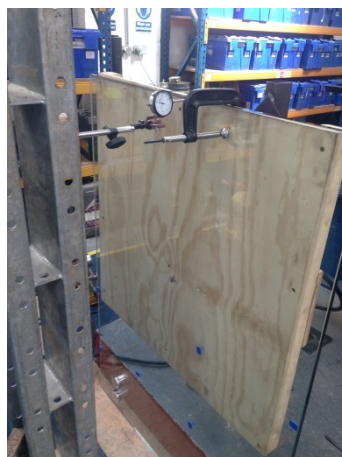
Figure 3: Setup for MS123 during uniformly distributed load test applied to the infill
