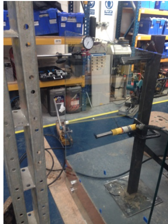
Figure 4: Setup for MS123 during point load test applied to the infill
