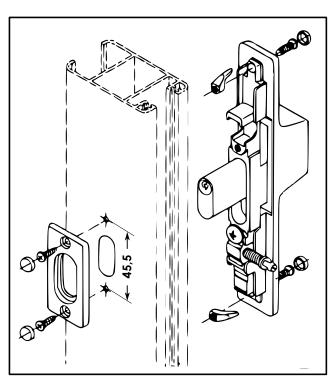
Create a hole on the external face of the profile and fit the locking cylinder rosette.
