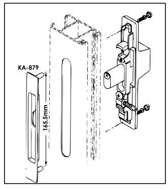
Additionally, you can fit the KA-879 opposite plate of the KA-370 & 380 instead of the locking cylinder rosette or in case you want to replace an old locking handle.
