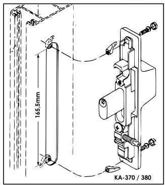
Create a hole, only on the internal face of the profile. Restraint the lock with the especially casted (hooks) components.
