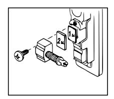
Use the correct spacers 1 & 2 to ensure the correct fit on any profiles depending on their width.
